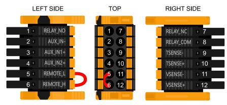
User I/O Connector is located on bottom left side of connection area, diagram shows 3 perspectives. Left Side - Top - Right Side
