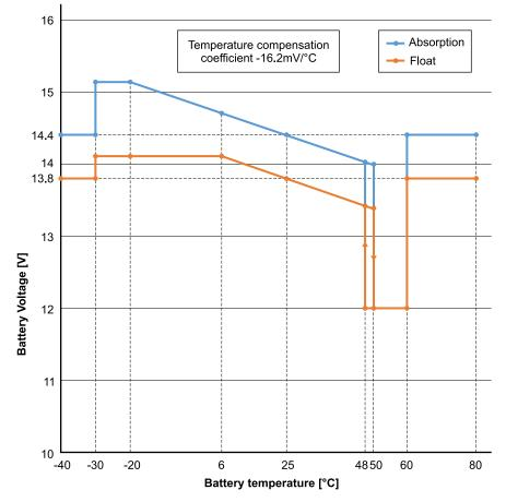
With a temperature sensor installed to the User I/O connection block; the actual battery temperature will be used for compensation; throughout the day.
