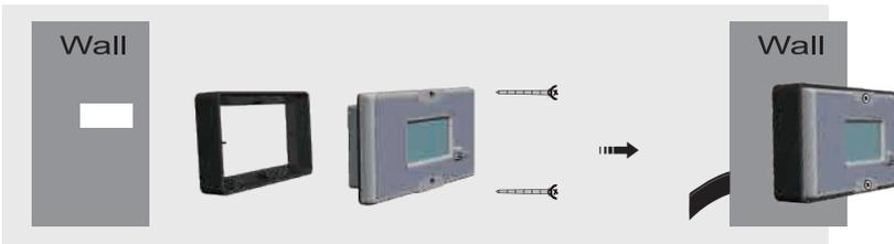
or ② With the frame and rear both, if the user just can screw the bracket on the wall, no hole for phone jack.
