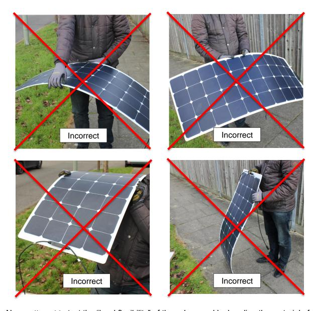
Never attempt to test the "local flexibility" of the solar panel by bending the material of the solar panel near the edges or in the corners. This can easily cause solar cell cracks.
