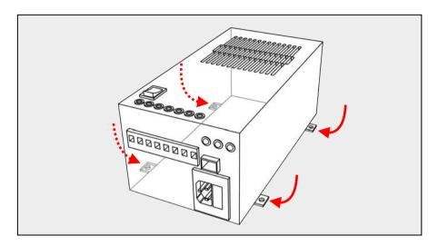
The ideal mounting position is smooth, well ventilated and not subject to overheating; avoid surfaces covered with fabric or carpet. Install the device as close as possible to the leisure batteries.
