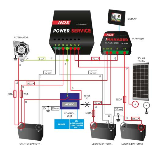
FOR CABLES LONGER THAN 2 METERS USE 16mm<sup>2</sup> CABLES The POWERSERVICE output must be connected to the common positive of the i-manager, in order to supply the two leisure batteries.
