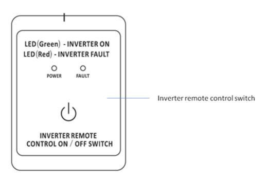
▲ Remote Control Usage: Please keep "OFF" position for switch of inverter, otherwise remote control function is invalid.
