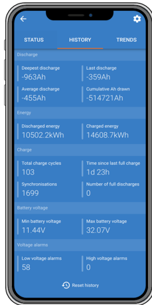
The VictronConnect app battery monitor history screen.
